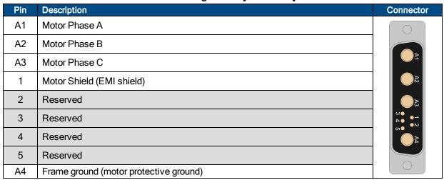
Table 3-2: 4-Pin Motor Connector Mating Connector
