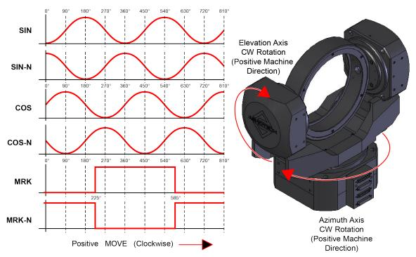
Figure 3-4: Analog Encoder Phasing Reference Diagram
