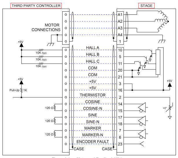
Figure 3-1: Motor and Feedback Wiring
