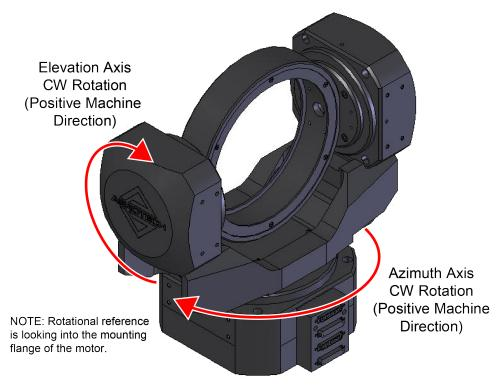
Figure 3-2: Machine Direction
