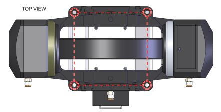
Figure 2-5: View of an AMG-LP Stage Showing Mounting Holes
