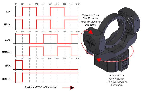
Figure 3-5: Encoder Phasing Reference Diagram (Standard)
