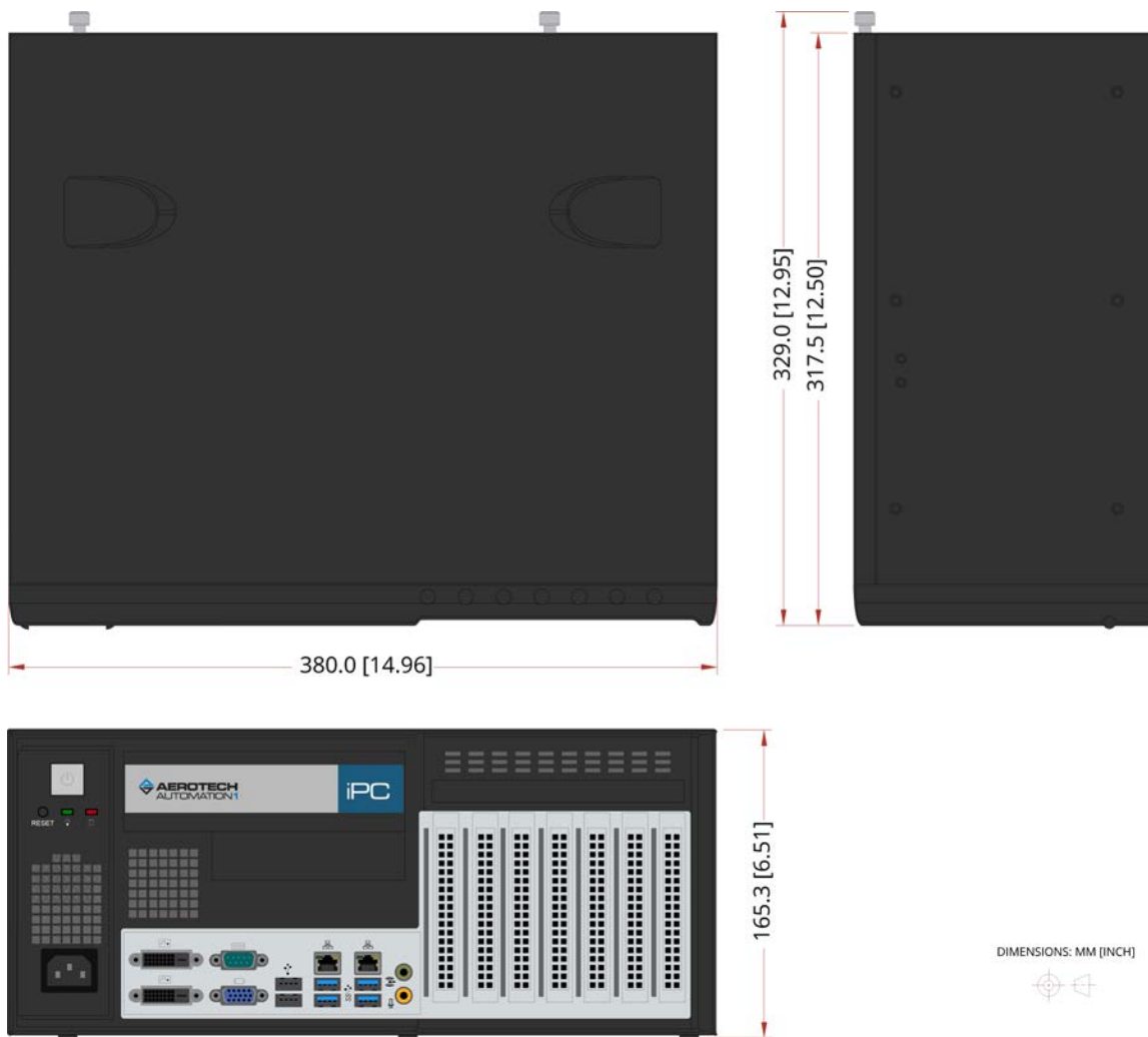
Figure 1-5: Desktop Computer Dimensions (-DT01)
