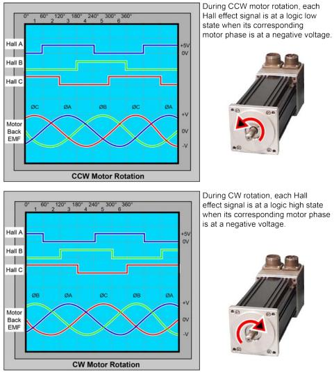
Figure 2-3: Hall Effect and Motor Phasing
