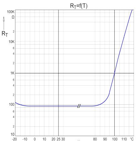
Figure 2-1: Typical Thermal Sensor Resistance as a Function of Temperature
