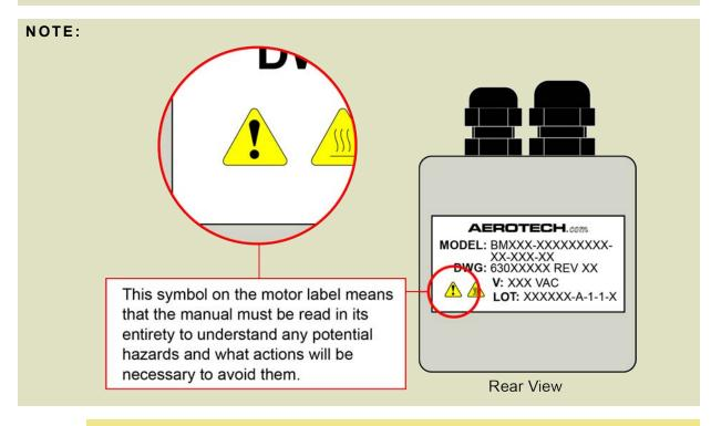
**DANGER:** The motor temperature can pose a burn hazard. Do not touch the motor until it has cooled sufficiently.
