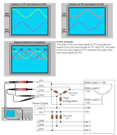
Figure 2-5: Motor Lead Phasing with Oscilloscope
