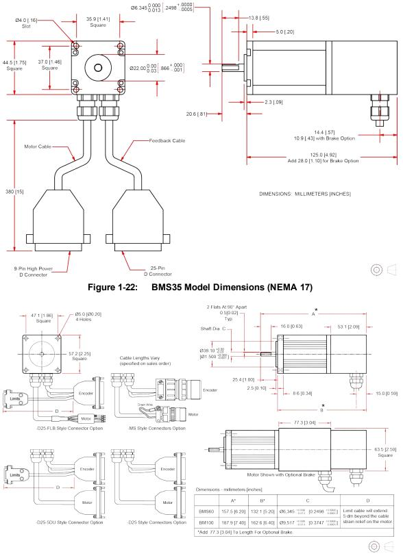
Figure 1-23: BMS60 and BMS100 Model Dimensions (NEMA 23)
