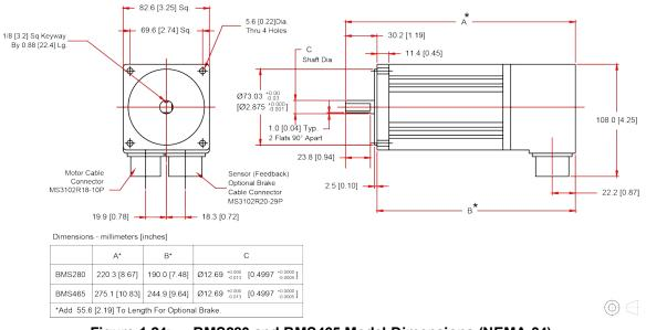
Figure 1-24: BMS280 and BMS465 Model Dimensions (NEMA 34)
