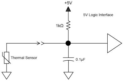
Figure 2-2: Typical Thermistor Interface Circuit
