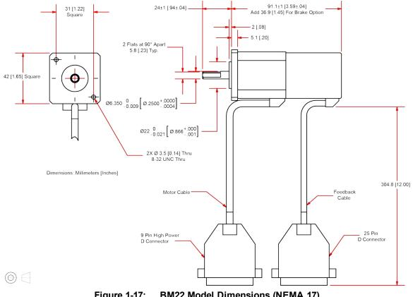
Figure 1-17: **BM22 Model Dimensions (NEMA 17)**
