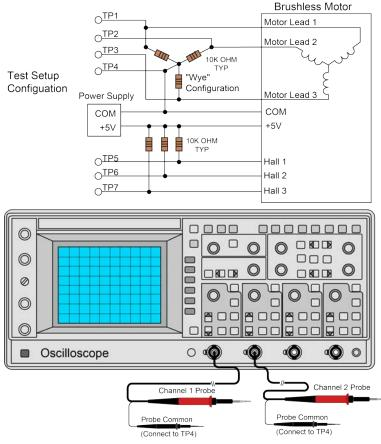
Figure 2-4: Test Setup Configuration
