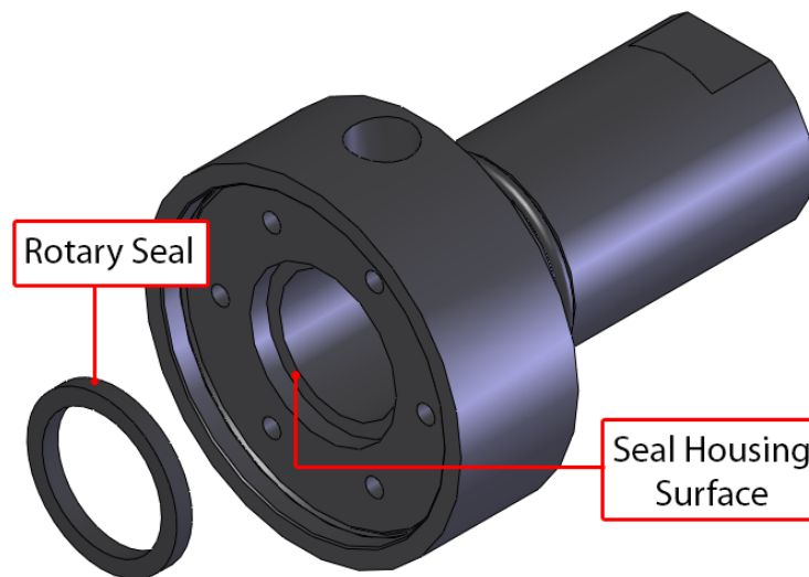
Figure 4-12: Seal Housing Location
