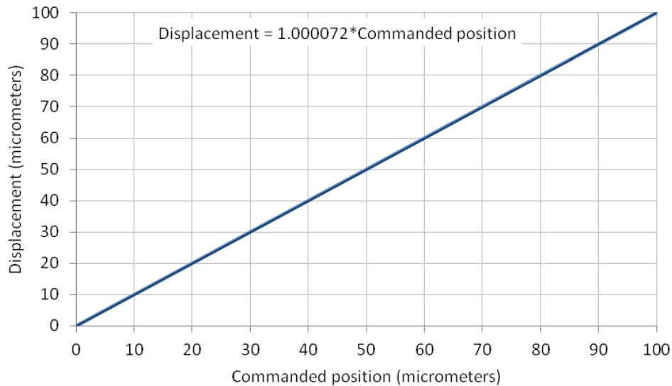
Figure C-7: Raw measurement results from an accuracy and linearity test of a 100 \mu\text{m} piezo stage
