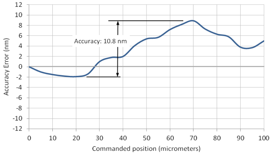
Figure C-8: Example accuracy error calculated from the measurement data shown in Figure C-7
