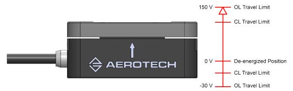
Figure 1-1: Single-Axis Stage Travel and Voltage Relationship
