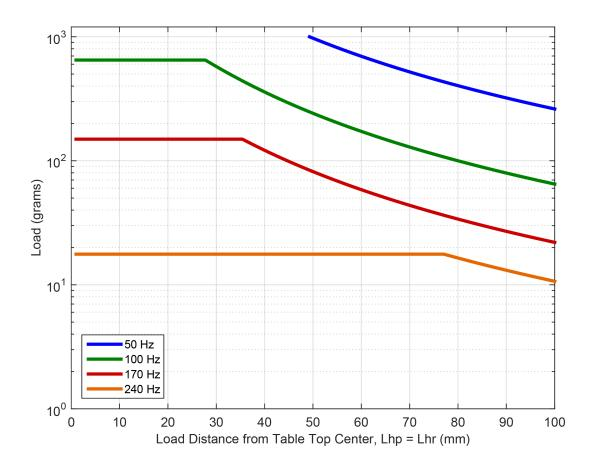
Figure 2-13: QNP60Z-500, 1st Natural Frequencies for Point Load Offset from Tabletop Center in HP Direction
