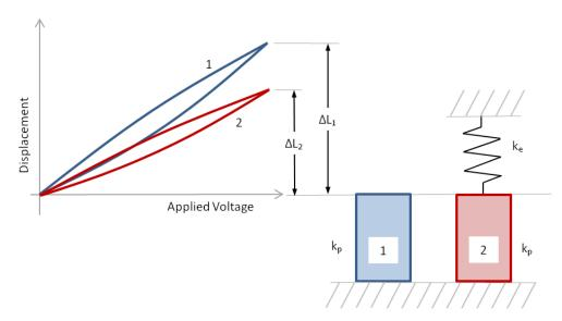
Figure C-5: Displacement of a piezo stage or actuator driving against an external spring of stiffness  ${\bf k}_{\!_{\rm P}}$
