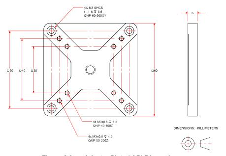
Figure 2-3: Adapter Plate (-AP) Dimensions
