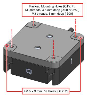
Figure 2-5: Mounting Hole Locations (Tabletop)
