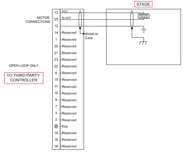
Figure 3-1: Piezo Actuator Wiring
