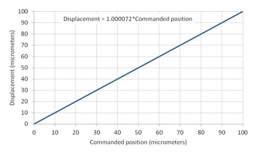
Figure C-7: Raw measurement results from an accuracy and linearity test of a 100 μm piezo stage
