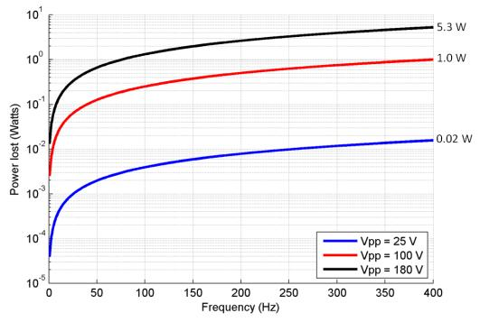
Figure C-6: Estimated power dissipated as a function of frequency and applied voltage for a typical piezo actuator with a 4 µF capacitance
