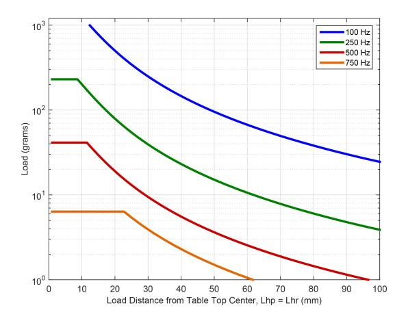
Figure 2-7: QNP40Z-100, 1st Natural Frequencies for Point Load Offset from Tabletop Center in HP Direction
