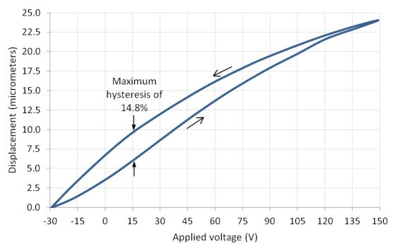
Figure C-2: Typical hysteresis curve of a piezoelectric stack actuator operating from -30V to +150V
