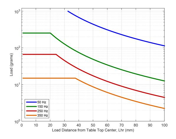
Figure 2-11: QNP50Z-250, 1st Natural Frequencies for Point Load Offset from Tabletop Center in HR Direction
