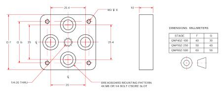
Figure 2-2: Mounting Plate (-MP) Dimensions
