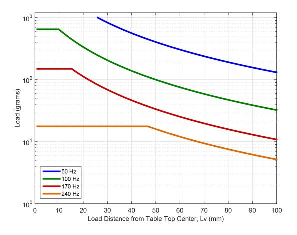
Figure 2-15: QNP60Z-500, 1st Natural Frequencies for Point Load Offset from Tabletop Center in V Direction
