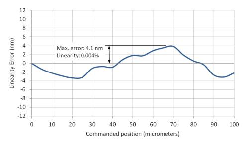
Figure C-9: Illustration showing how linearity is calculated based on measurement data taken from a 100 µm piezo nanopositioning stage
