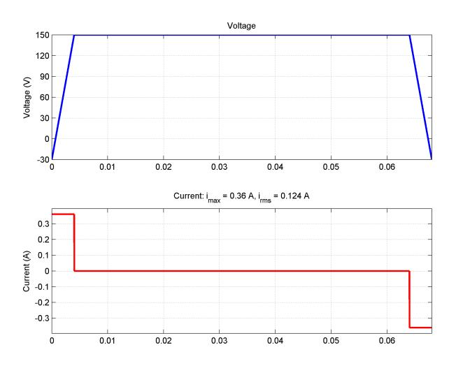
Figure C-12: Voltage and current waveforms for the profile commanded in Example 2
