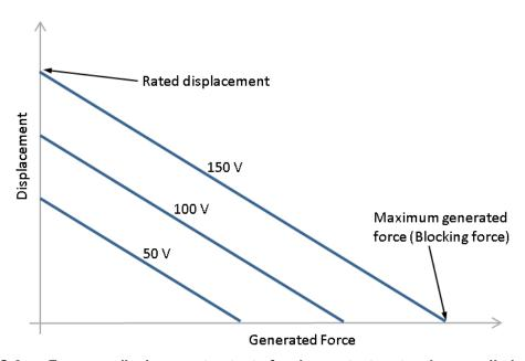
Figure C-3: Force vs. displacement output of a piezo actuator at various applied voltages
