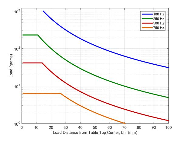
Figure 2-8: QNP40Z-100, 1st Natural Frequencies for Point Load Offset from Tabletop Center in HR Direction
