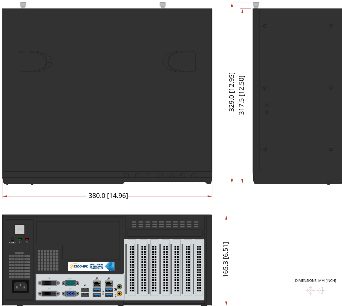
Figure 1-5: Desktop Computer Dimensions (-DT01)
