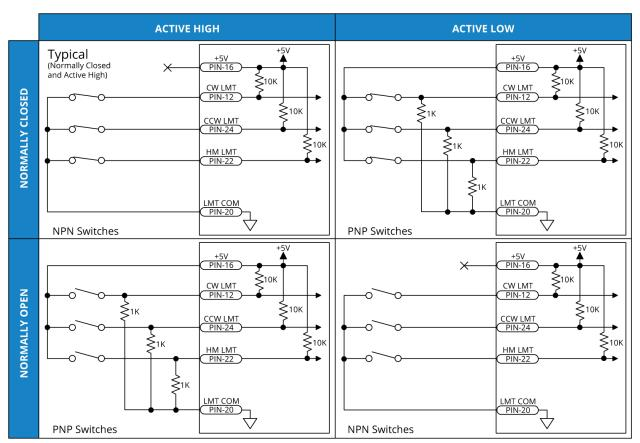
Figure 2-21: End of Travel and Home Limit Input Connections
