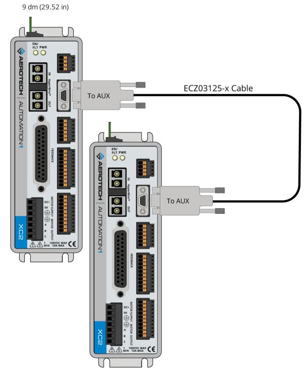
Figure 4-4: Dual-Axis PSO Cable Connection
