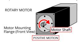
Figure 2-9: Positive Motor Direction
