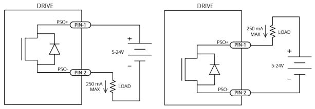
Figure 3-2: PSO Output Sources Current
