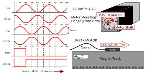
Figure 2-14: Sine Wave Encoder Phasing Reference Diagram
