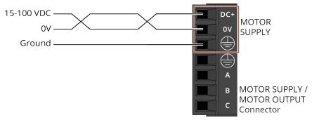
Figure 2-2: Motor Supply Connections
