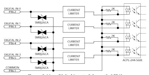
Figure 3-11: Digital Inputs Schematic [-EB1]
