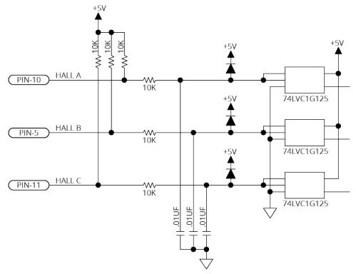
Figure 2-18: Hall-Effect Inputs Schematic (Feedback Connector)
