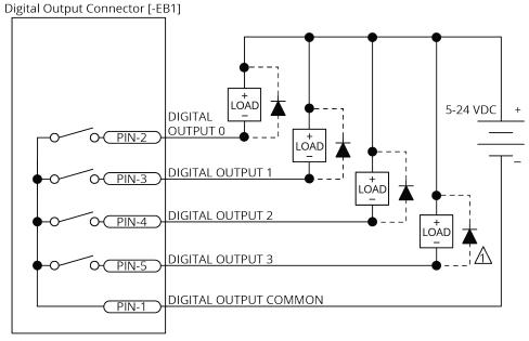
DIODE REQUIRED ON EACH OUTPUT THAT DRIVES AN INDUCTIVE DEVICE (COIL), SUCH AS A RELAY.
