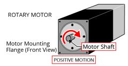
Figure 2-11: Positive Motor Direction
