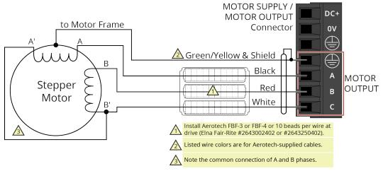
Figure 2-10: Stepper Motor Configuration
