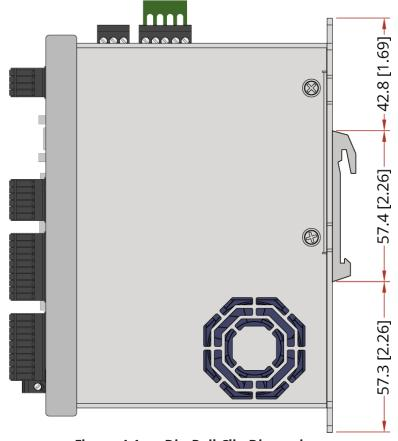
Figure 4-1: Din Rail Clip Dimensions
