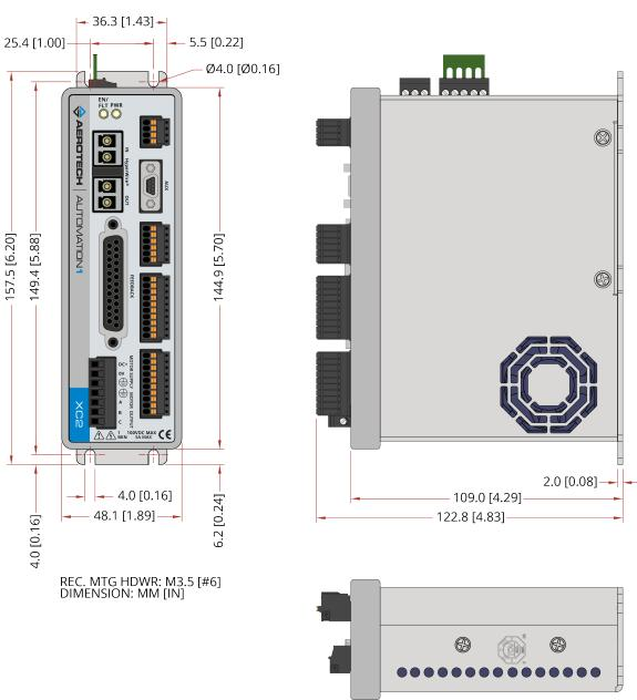
Figure 1-4: Dimensions [-EB1]
