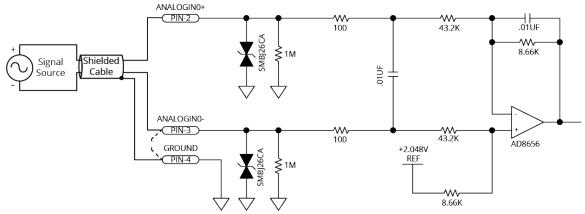
Figure 3-7: Analog Input Schematic [-EB1]
