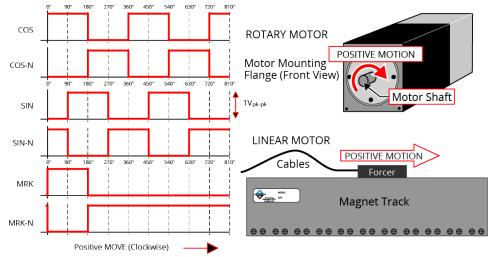
Figure 2-16: Encoder Phasing Reference Diagram (Standard)
