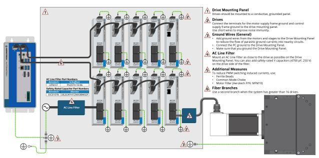
Figure 2-27: System Wiring Drawing (Best Practice)
