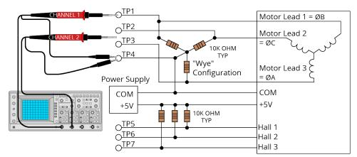
Figure 2-6: Brushless Motor Phasing Oscilloscope Example
