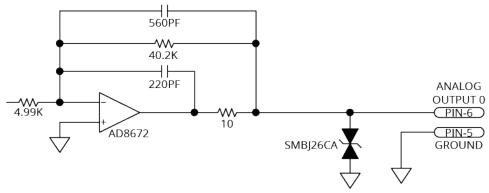
Figure 3-6: Analog Output Schematic [-EB1]
