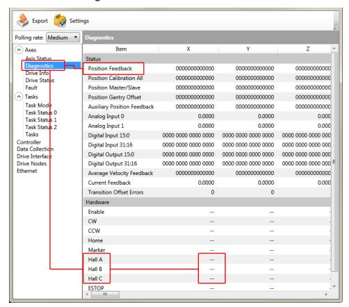
Figure 2-5: Encoder and Hall Signal Diagnostics
