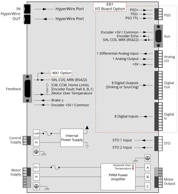
Figure 1-2: Functional Diagram
