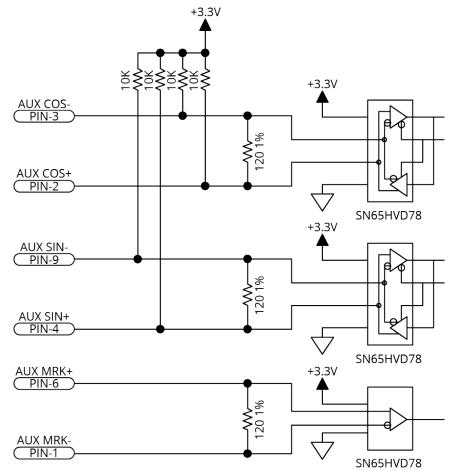
Figure 3-5: Square Wave Encoder Interface (Aux Connector)
