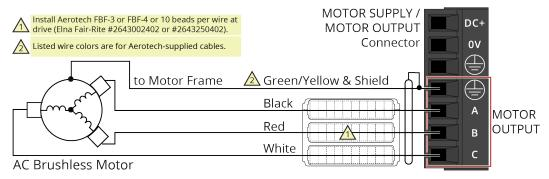
Figure 2-3: Brushless Motor Configuration
