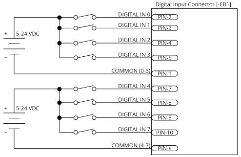
Figure 3-12: Digital Inputs Connected to Current Sourcing (PNP) Devices [-EB1]
