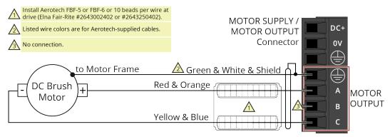
Figure 2-8: DC Brush Motor Configuration
