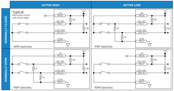
Figure 2-8: End of Travel Limit Input Connections
