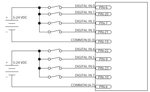
Figure 2-25: Digital Inputs Connected to Current Sourcing (PNP) Devices
