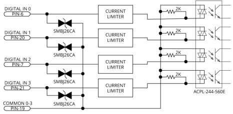
Figure 2-24: Digital Inputs Schematic
