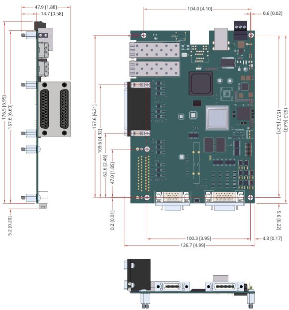
Figure 1-6: Dimensions [-2P2 (OEM 2-Axis)]
