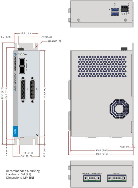
Figure 1-4: Dimensions [-2P1 (Standard 2-Axis)]
