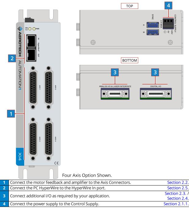
Figure 1: Installation Connection Overview (4 Axis Shown)
