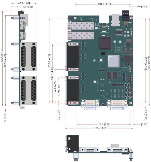
Figure 1-7: Dimensions [-4P2 (OEM 4-Axis)]
