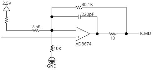
Figure 2-2: Current Command Output Schematic
