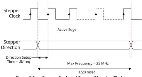
Figure 2-3: Stepper Clock and Stepper Direction Timing
