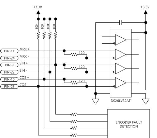
Figure 2-13: Square Wave Encoder Schematic (Axis Connector)
