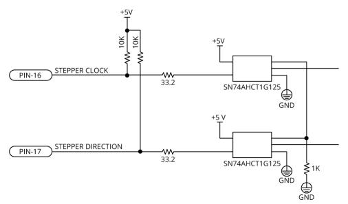
Figure 2-4: Stepper Clock and Stepper Direction Output Schematic
