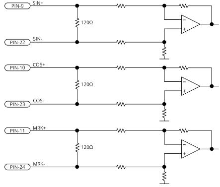
Figure 2-16: Sine Wave Encoder Schematic (Axis Connector)
