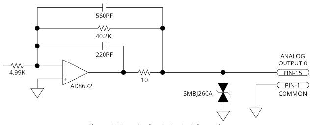
Figure 2-30: Analog Outputs Schematic
