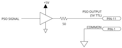
Figure 2-28: PSO TTL Outputs Schematic
