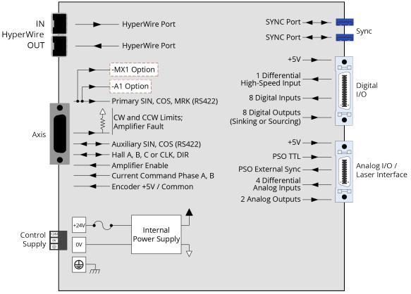
Figure 1-3: Functional Diagram
