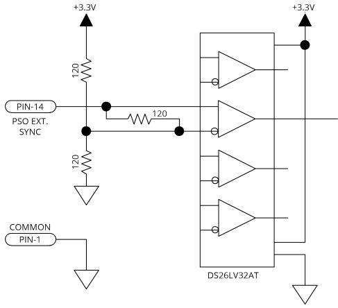
Figure 2-29: PSO External Sync Input Schematic
