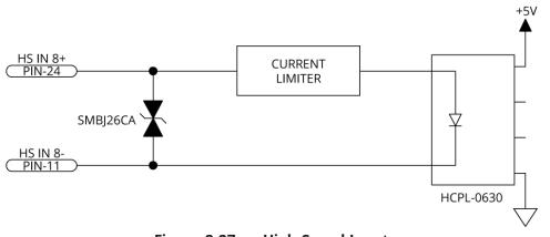
Figure 2-27: High-Speed Input
