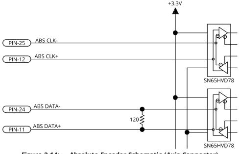
Figure 2-14: Absolute Encoder Schematic (Axis Connector)
