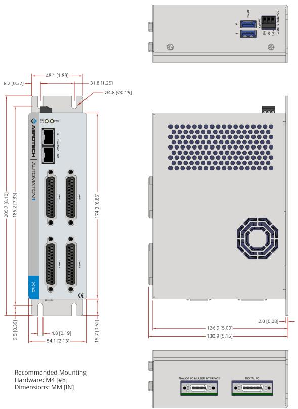
Figure 1-5: Dimensions [-4P1 (Standard 4-Axis)]
