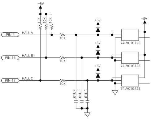
Figure 2-5: Hall-Effect Inputs Schematic
