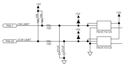
Figure 2-9: End of Travel Limit Input Schematic
