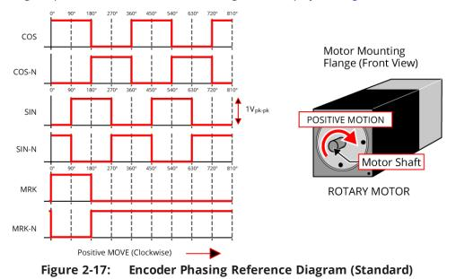
**IMPORTANT**: Encoder manufacturers may refer to the encoder signals as A, B, and Z. The proper phase relationship between signals is shown in Figure 2-17.
