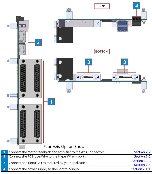
Figure 2: Installation Connection Overview (4 Axis OEM Shown)
