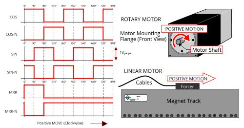
Figure 2-17: Encoder Phasing Reference Diagram (Standard)
