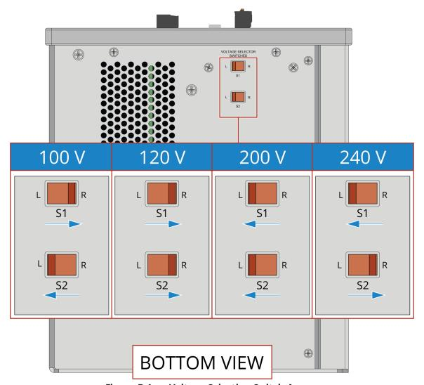
Figure B-1: Voltage Selection Switch Access
