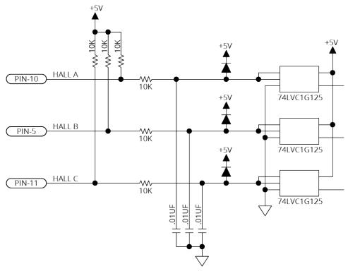
Figure 2-19: Hall-Effect Inputs Schematic (Feedback Connector)
