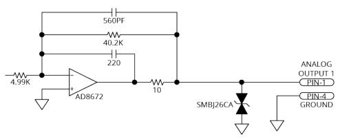
Figure 3-8: Analog Output Typical Connection [-EB1]
