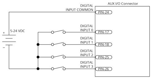
Figure 2-38: Digital Inputs Connected to Current Sinking Devices
