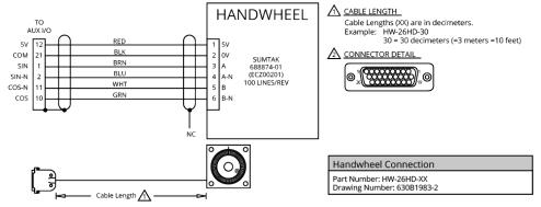
Figure 4-3: Handwheel Interconnection to Aux I/O Connector
