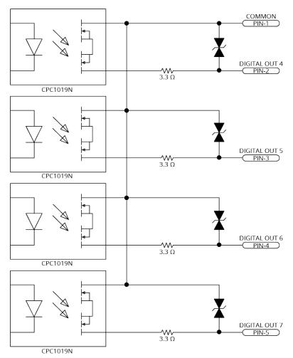
Figure 3-2: Digital Outputs Schematic [-EB1]
