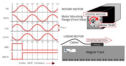
Figure 2-15: Sine Wave Encoder Phasing Reference Diagram
