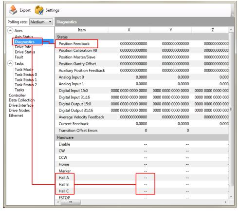
Figure 2-5: Encoder and Hall Signal Diagnostics
