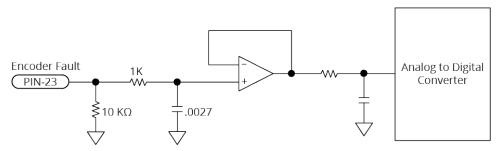
Figure 2-21: Encoder Fault Input Schematic (Feedback Connector)
