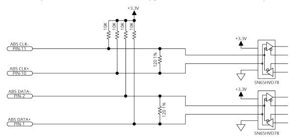
Figure 2-29: Absolute Encoder Schematic (Auxiliary I/O Connector)
