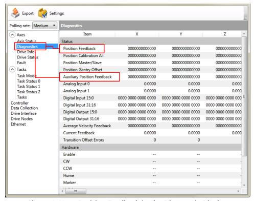
Figure 2-18: Position Feedback in the Diagnostic Display
