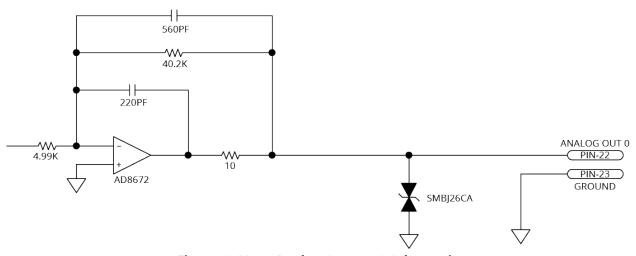
Figure 2-40: Analog Output 0 Schematic
