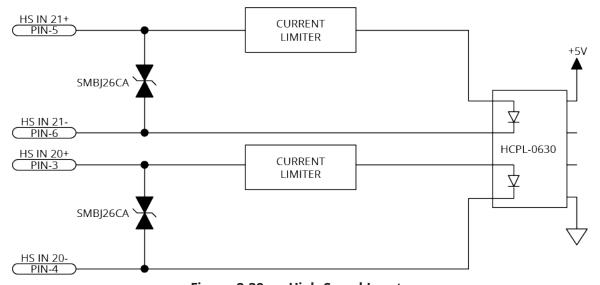
Figure 2-39: High-Speed Inputs
