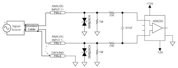
Figure 3-9: Analog Input Typical Connection [-EB1]
