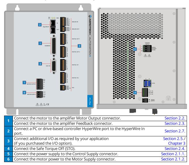
Figure 1: Installation Connection Overview
