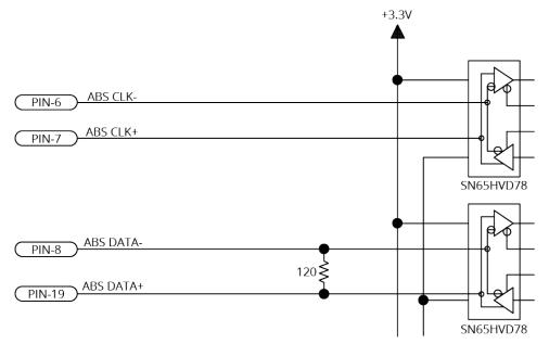
Figure 2-14: Absolute Encoder Schematic (Feedback Connector)
