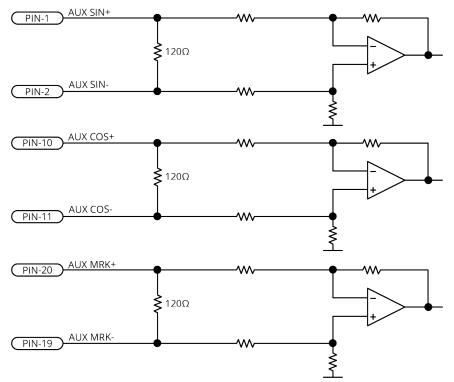
Figure 2-31: Sine Wave Encoder Schematic (Auxiliary I/O Connector)
