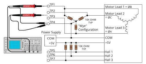
Figure 2-6: Brushless Motor Phasing Oscilloscope Example
