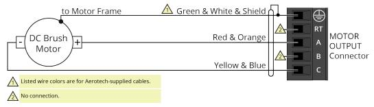
Figure 2-8: DC Brush Motor Configuration
