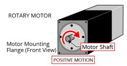
Figure 2-10: Positive Motor Direction
