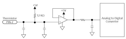
Figure 2-20: Thermistor Input Schematic (Feedback Connector)
