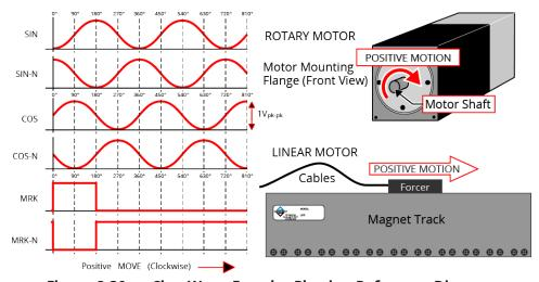
Figure 2-30: Sine Wave Encoder Phasing Reference Diagram
