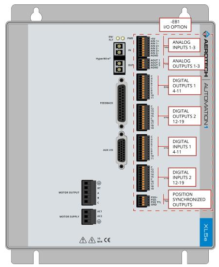
Figure 3-1: XL5e with -EB1 I/O Option Board Connectors
