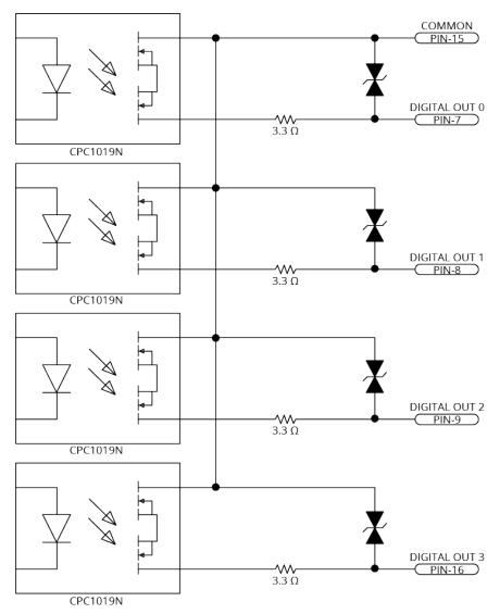
Figure 2-33: Digital Output Schematic (Aux I/O Connector)
