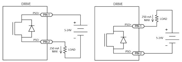
Figure 3-10: PSO Output Sources Current
