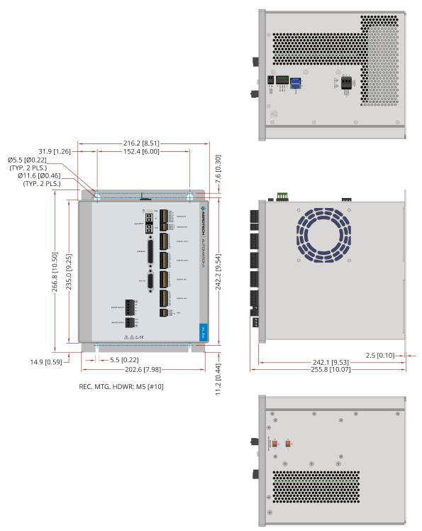
Figure 1-4: Dimensions [-EB1]
