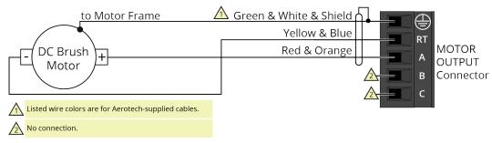
Figure 2-9: DC Brush Motor Configuration
