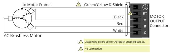
Figure 2-3: Brushless Motor Configuration
