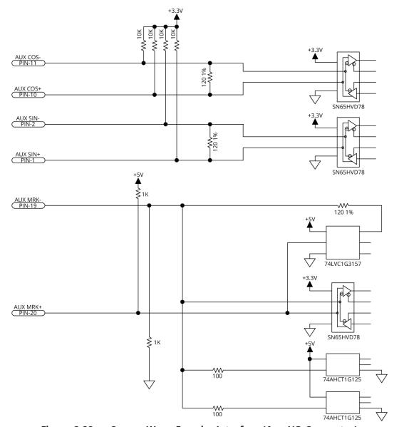
Figure 2-28: Square Wave Encoder Interface (Aux I/O Connector)
