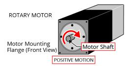
Figure 2-12: Positive Motor Direction
