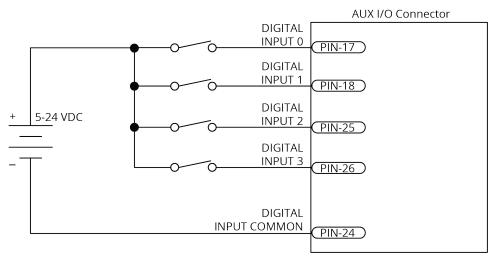
Figure 2-37: Digital Inputs Connected to Current Sourcing Devices
