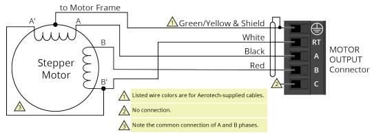
Figure 2-11: Stepper Motor Configuration
