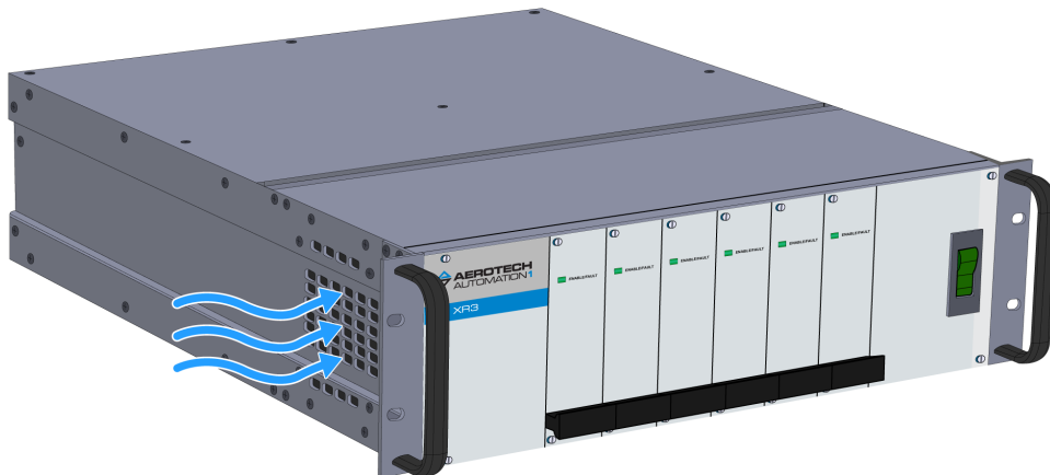
Figure 2-47: -C0 Fan Location and Direction of Air Flow
