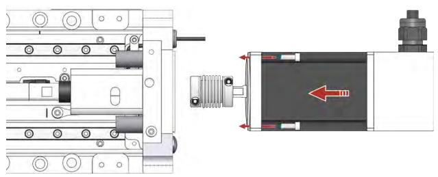
Figure 4-5: Attach the Motor the Stage
