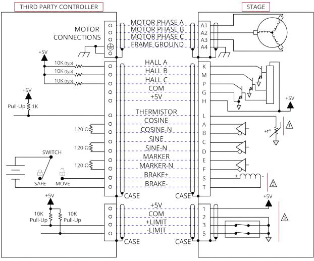
Thermistor is only available on BMS motors. 🔬 Limit options are factory-configured as normally closed or normally open.
