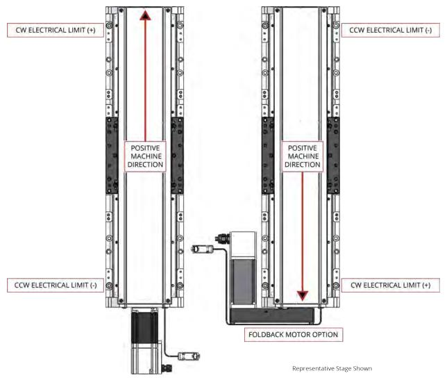
Figure 3-3: Machine Direction
