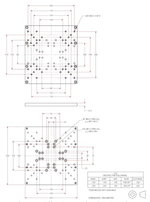
Figure 2-3: Tabletop Accessory Dimensions (-TT3 Option)
