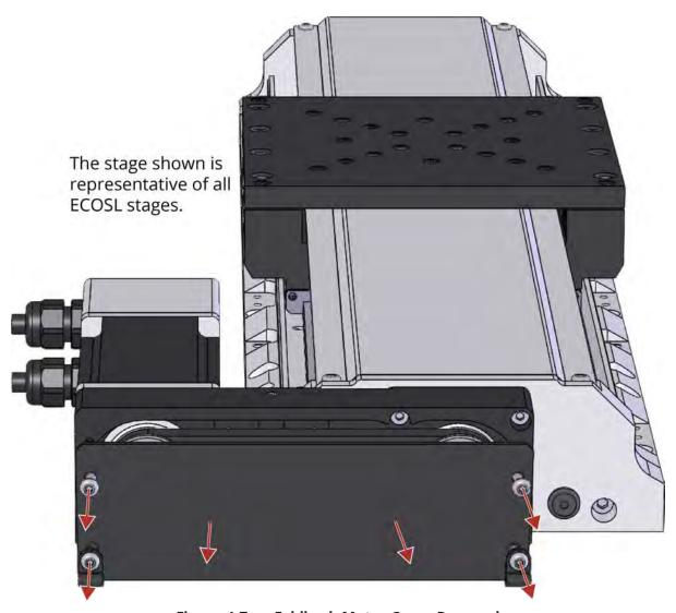
Figure 4-7: Foldback Motor Cover Removal
