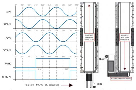
Figure 3-6: Encoder Phasing Reference Diagram (Analog/Sine Wave)
