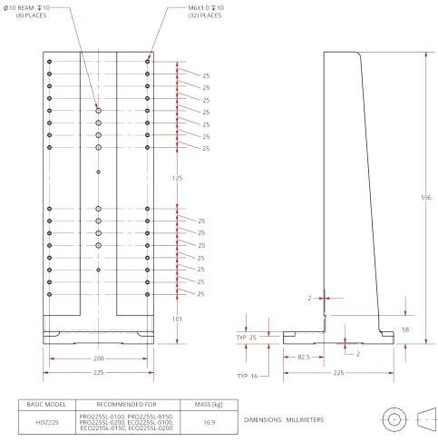
Figure 2-4: Z-Axis Bracket Dimensions
