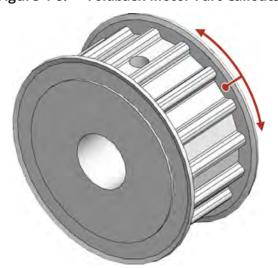
Figure 4-9: Lubricate the Pulley Flanges
