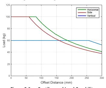
Figure 2-6: Cantilevered Load Capability
