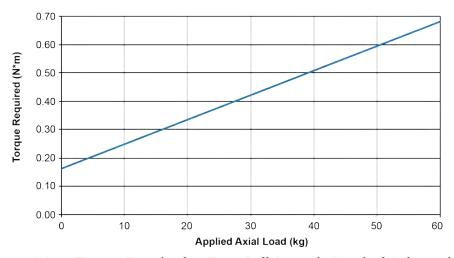
Figure 2-8: Torque Required to Turn Ball Screw in Vertical Orientation
