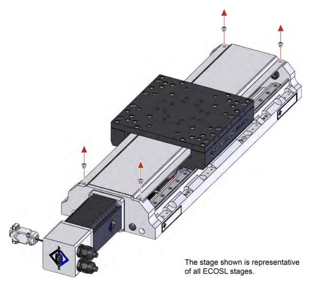
Figure 4-1: Hardcover Screw Removal
