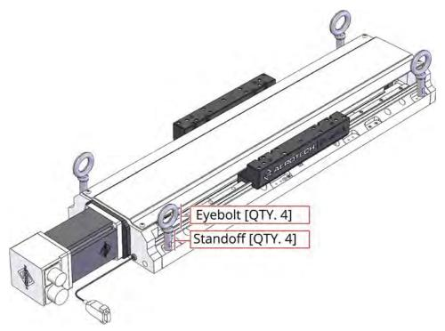
Figure 2-1: Lifting Features
