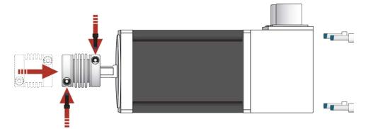
Figure 4-5: Attach the Coupling Adapter to the Motor Shaft
