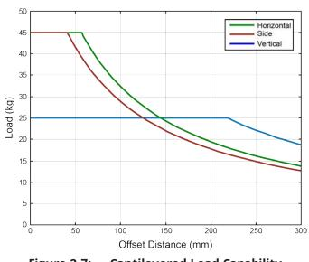
Figure 2-7: Cantilevered Load Capability
