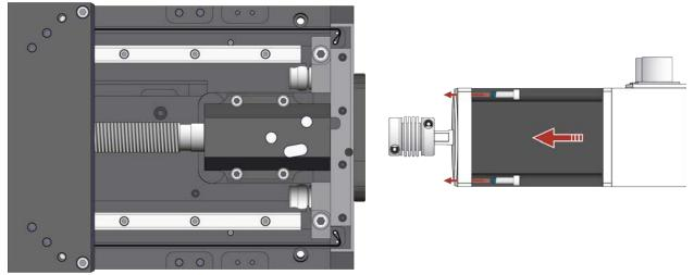
Figure 4-6: Attach the Motor the Stage
