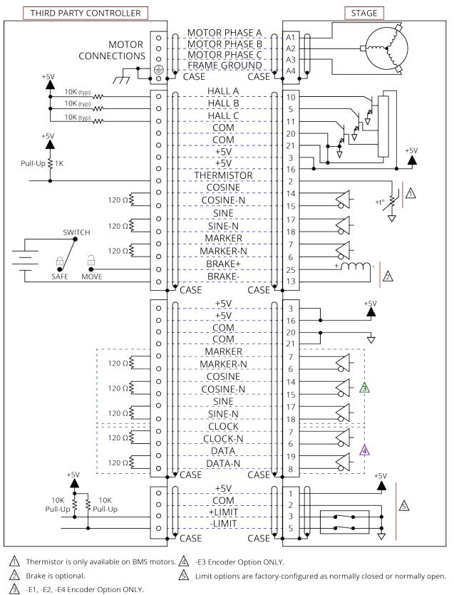
Figure 3-2: Brushless Motor and Feedback Wiring [-SLE Option]
