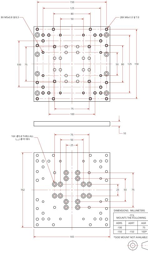
Figure 2-4: Tabletop Accessory Dimensions (-TT3 Option)
