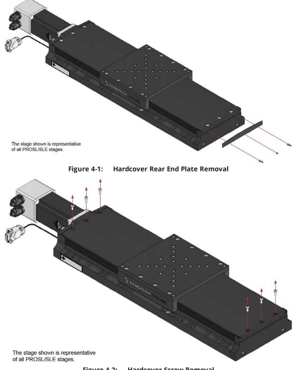
Figure 4-2: Hardcover Screw Removal
