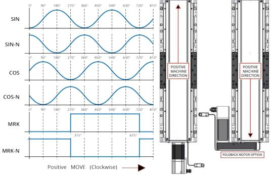
Figure 3-6: Encoder Phasing Reference Diagram (Analog/Sine Wave)
