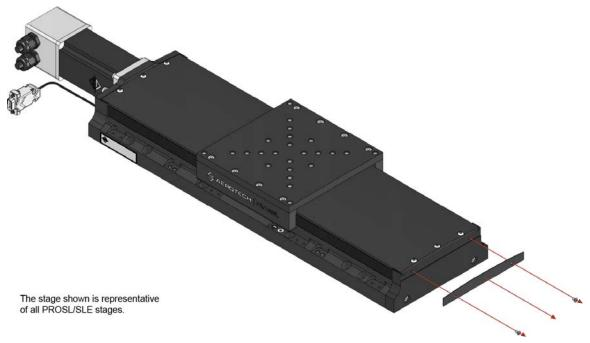
Figure 4-1: Hardcover Rear End Plate Removal
