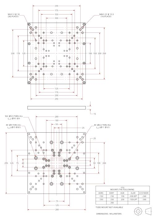
Figure 2-4: Tabletop Accessory Dimensions (-TT3 Option)
