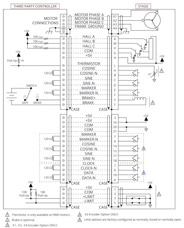
Figure 3-2: Brushless Motor and Feedback Wiring [-SLE Option]
