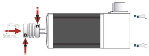
Figure 4-5: Attach the Coupling Adapter to the Motor Shaft
