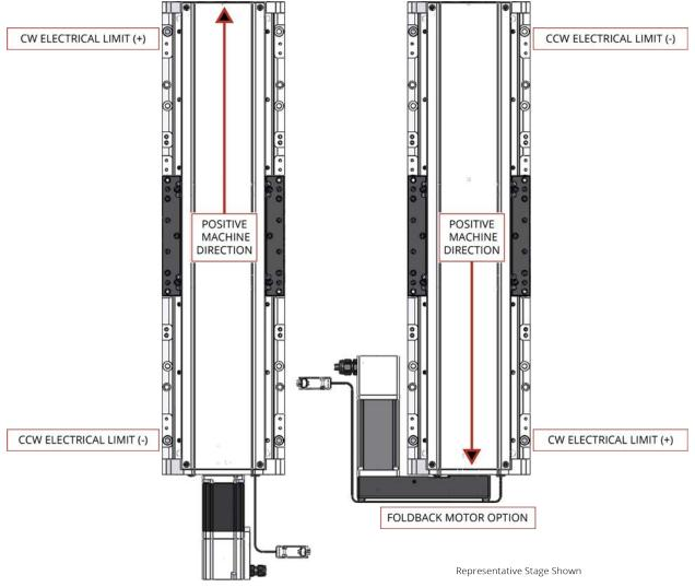
Figure 3-3: Machine Direction
