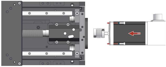
Figure 4-6: Attach the Motor the Stage
