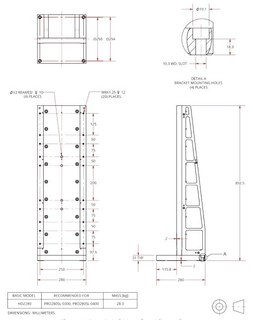
Figure 2-5: Z-Axis Bracket Dimensions
