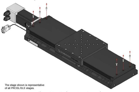
Figure 4-2: Hardcover Screw Removal
