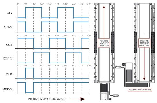
Figure 3-5: Encoder Phasing Reference Diagram (Standard/Square Wave)
