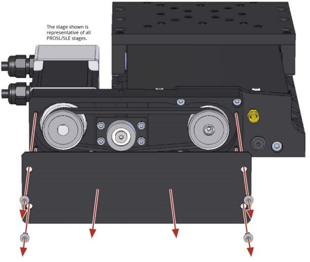
Figure 4-8: Foldback Motor Cover Removal
