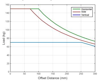
Figure 2-7: Cantilevered Load Capability
