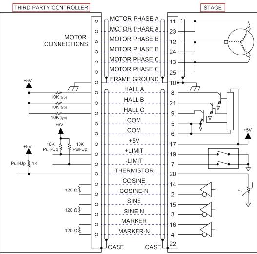
Figure 3-1: ANT95L Motor and Feedback Wiring
