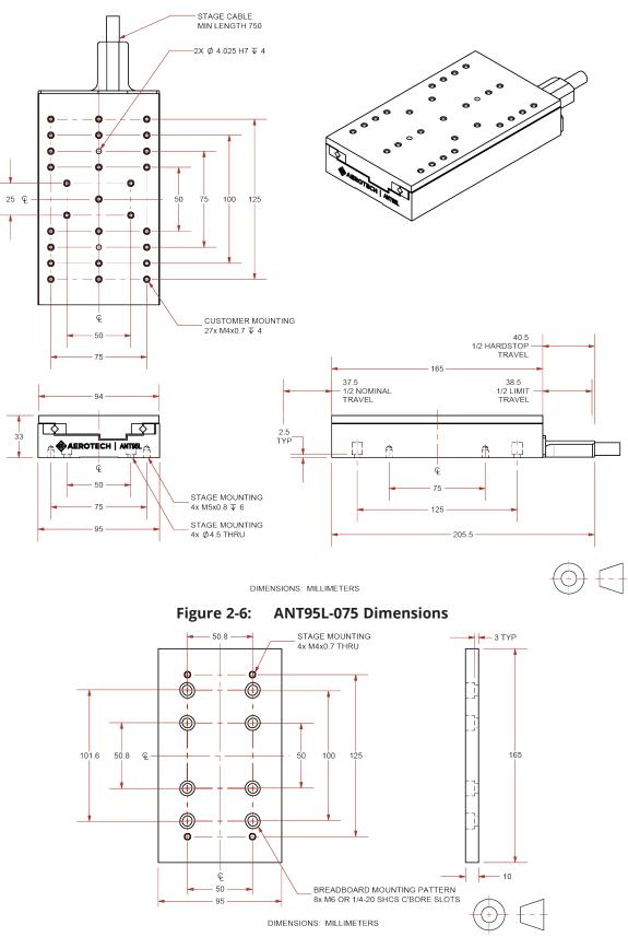
Figure 2-7: ANT95L-075 Mounting Plate Dimensions
