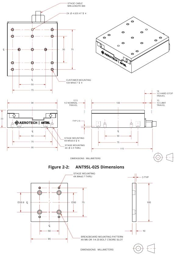
Figure 2-3: ANT95L-025 Mounting Plate Dimensions
