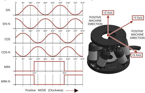
Figure 3-5: Encoder Phasing Reference Diagram (Standard)
