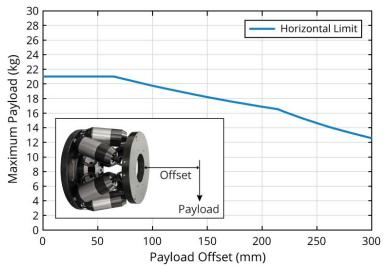
Figure 2-6: HEX300-230HL Inverted Load Capabilities
