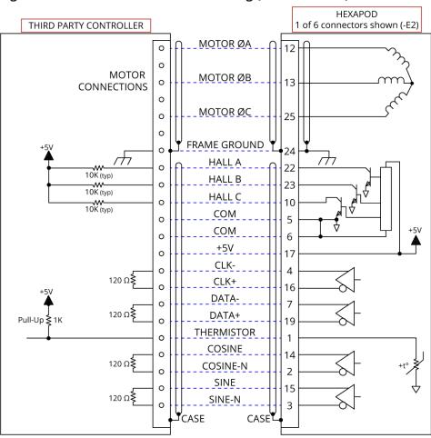
Figure 3-2: Motor and Feedback Wiring (-E2 Connector)
