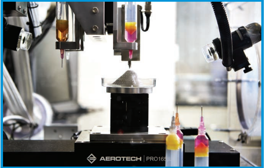
Aerotech motion products are already being used in a variety of additive manufacturing applications. This application, at The Wake Forest Institute for Regenerative Medicine, shows a 3D printer that can construct nose scaffolding – simultaneously embedding it with cells that will later grow into tissue.
