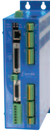
Ensemble CP Width: 63.5 mm Height: 198.2 mm
