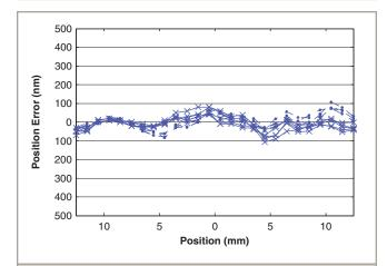
ANT95L-025PLUS accuracy and repeatability. This multiple test run over an extended period of time shows the high level of system accuracy and repeatability.
