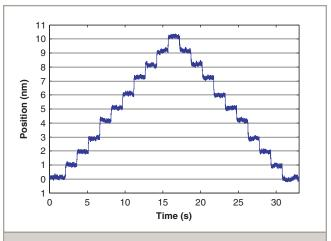
ANT95L 1 nm step plot. Best-in-class resolution and exceptional inposition stability for large travel stages.
