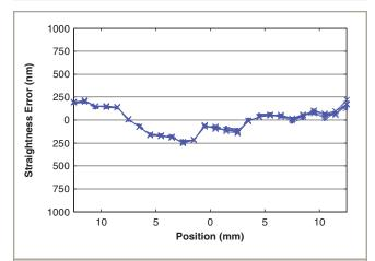
ANT95L-025PLUS straightness error, five runs, bi-directional. Exceptional and highly repeatable – five times more accurate than the stated specification.
