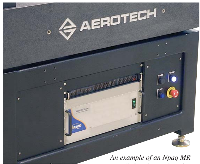
Npaq MR is a 3U, 19-inch rack-mount 4- or 8-axis drive rack.
