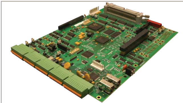
A3200-OEM control board (2 or 4 axis).
