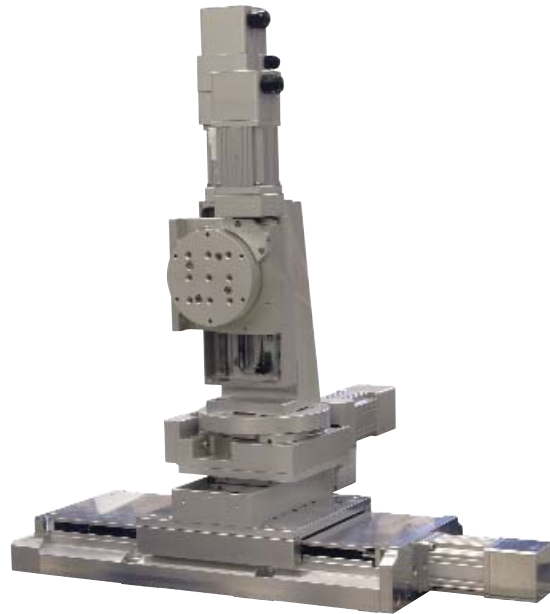
Satellite Component Testing. Standard vacuum ( 10^{-6} torr), 5-axis positioning system incorporating two worm-drive rotary stages and three ball-screw-driven linear stages.
