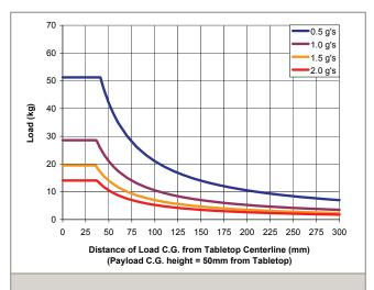
Yaw offsets with payload C.O.G. 50 mm above the tabletop.
