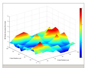
QNP2-100XYA-100-C two-dimensional accuracy error measured with an external laser interferometer targeting a two-sided optical square. The results show the nanometerlevel positioning performance capability of the QNP2 series over the complete XY travel.
