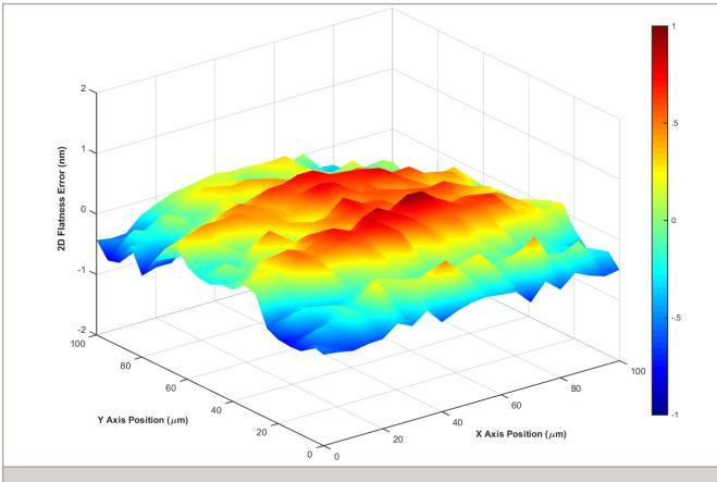
*QNP2-100XYA-100-C* two-dimensional flatness of 1.5 nm over the full XY travel. The results show the outstanding geometric performance of the QNP2 series.
