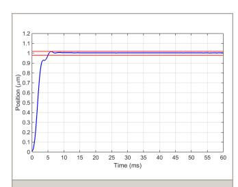
QNP2-100XYA-100-C single-axis move-and-settle plot of 5.1 ms for a 1  $\mu$ m move with a 120 gram load and  $\pm$ 20 nm settle window illustrating the high-throughput capability of the QNP2 series.
