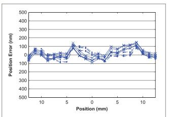
ANT95XY-025-PLUS accuracy and repeatability, five runs, bi-directional for the X (lower) axis. The total accuracy of 240 nm over 25 mm travel is significantly better than other offerings and half of its stated specification.
