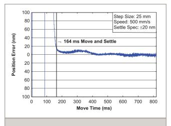
ANT95XY-025-PLUS step and settle performance at full travel and 1 kg payload for the X (lower) axis. Industry-best settling times significantly improve throughput for most applications.
