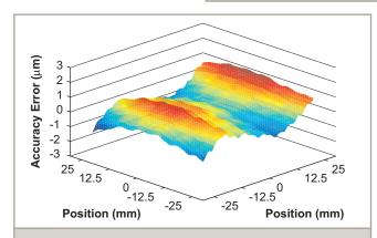
ANT95XY-050 2D accuracy plot showing planar accuracy error including straightness, orthogonality, and stage yawing.
