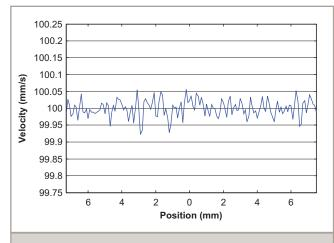
ANT95XY-025-PLUS velocity performance at 100 mm/s and 1 kg payload for the X (lower) axis. This outstanding speed stability enhances most scanning or laser machining applications.
