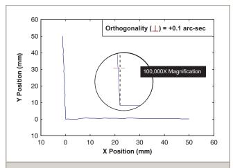
ANT95XY-050-ULTRA orthogonality. The inset is magnified 100,000X for clarity. The ULTRA model orthogonality is a twenty-fold improvement over the BASE model orthogonality.
