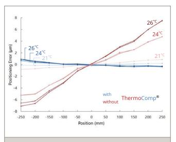
Measurement data showing successful compensation of thermal related positioning errors at several temperatures using the ThermoComp feature. Results are typical of stage performance with and without ThermoComp.
