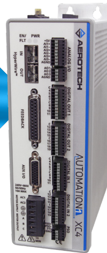
Aerotech's XC4 next generation panel-mount controller with high-speed optical HyperWire communication bus.
