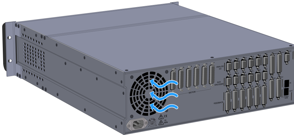
Figure 2-48: Location of the Rear Fan and Air Flow
