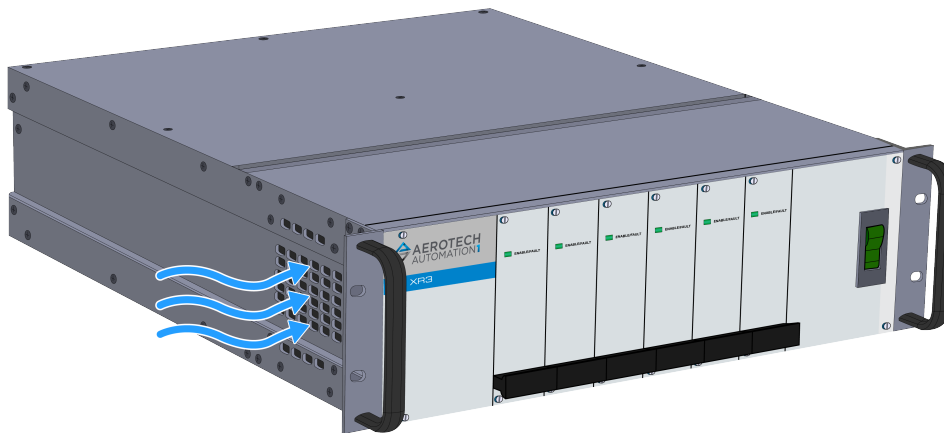
Figure 2-49: -C0 Fan Location and Direction of Air Flow
