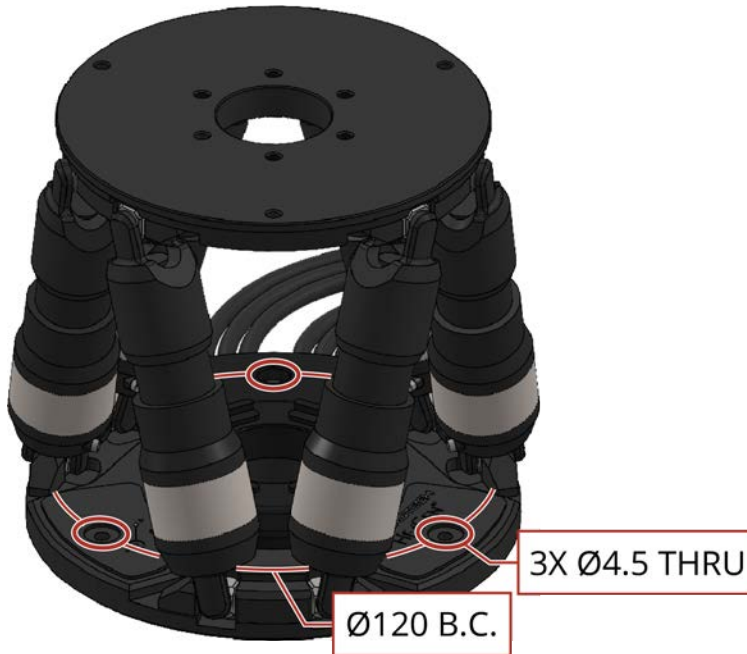
Figure 2-2: Mounting Hole Locations
