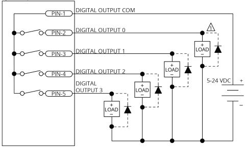
A DIODE REQUIRED ON EACH OUTPUT THAT DRIVES AN INDUCTIVE DEVICE (COIL), SUCH AS A RELAY.
