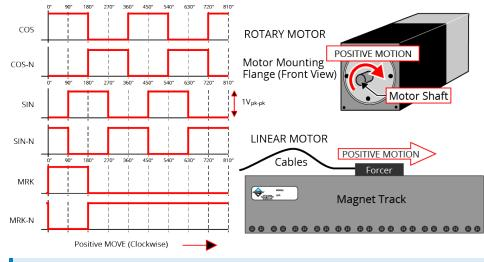
Figure 2-16: Encoder Phasing Reference Diagram (Standard)
