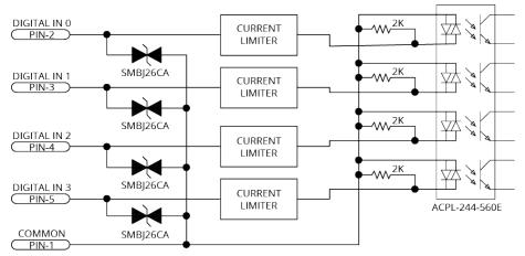
Each bank of four inputs must be connected in an all sourcing or all sinking configuration.
