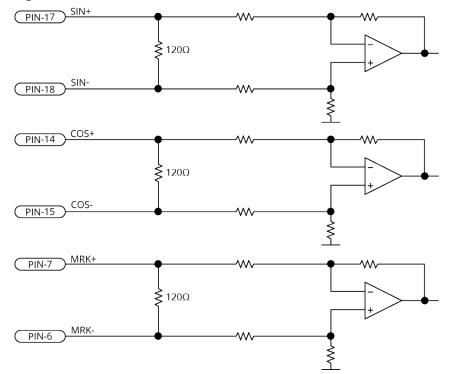
Figure 2-15: Sine Wave Encoder Schematic (Feedback Connector)
