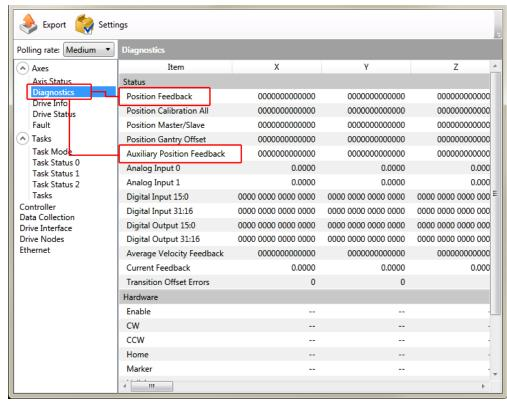
Figure 2-17: Position Feedback in the Diagnostic Display
