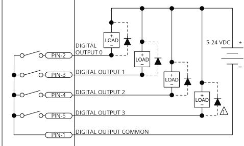
1 DIODE REQUIRED ON EACH OUTPUT THAT DRIVES AN INDUCTIVE DEVICE (COIL), SUCH AS A RELAY.
